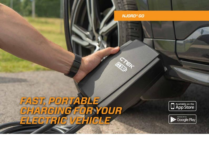
NJORD® GO is a portable 11kW EV charger\* that gives you fast, reliable Electric Vehicle (EV) charging at home, or when you're on the move. The charger can be used with the CTEK APP to unlock additional features, for complete charging control and monitoring via your mobile phone.
